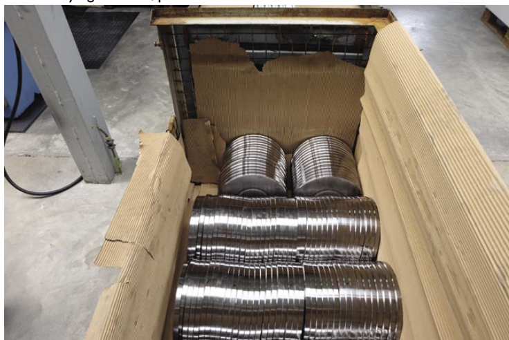
Aluminium platters sit in shiny lines after being turned on metal lathes.
